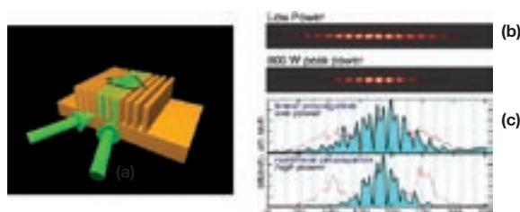
▲ (a) Experimental head-on geometry. (b,c) Experimental results for the generation of gap solitons in weakly coupled waveguide arrays and optically-induced photonic lattices. Shown are: (b) photographs of the beams at the array output, and (c) the output beam profiles for light propagating in optically-induced nonlinear lattices, where shading marks the minima of the refractive.
