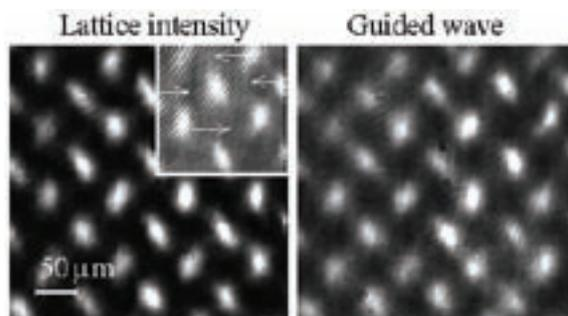
▲ Left: Example of a two-dimensional optically-induced photonic lattice with a vortex-like phase structure. Right: probe beam lattices guided by the photonic structure.
