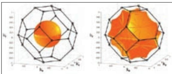
▲ Calculated iso-energy surfaces for a woodpile structure having a contrast in refractive indices of 1.56 for frequencies far below the bandgap (left image, behaves like a homogeneous medium) and slightly above the bandgap (right image, strong superprism effects).
