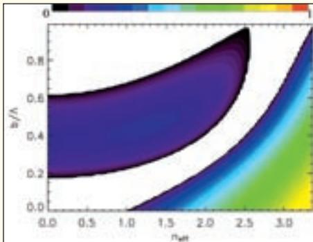
Summary of the properties of light propagating in a one-dimensional photonic crystal, consisting of silicon and air. Shown on the axes are the fill fraction of silicon, and the effective index of the mode. The coloured regions indicate the positions of bandgaps, with the colour coding showing the rate at which the field decays. The optimum configuration occurs for low, but nonzero silicon fraction and large effective index.
