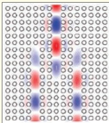
◀ An efficient photonic crystal Y coupler, as used in a Mach-Zehnder interferometer, that can achieve a transmittance exceeding 99.5% over a very wide wavelength range.
