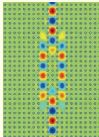
◀ Electric field plot showing the 'on' state of a symmetric photonic crystal M-Z interferometer with two coupled y-junctions. When a phase delay is introduced into one arm, anti-symmetric field components are recirculated through the interferometer producing resonance effects and a considerably sharper phase response than in conventional M-Z Interferometers.
