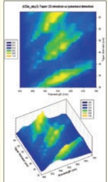
Reflectance spectra of dye inside a tapered microstructured optical fibre.
