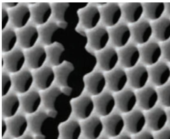
▲ Image of a broken section of the Photonic crystal lattice.
