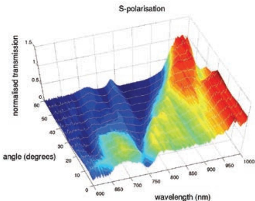
▲ The optical transmission of the lattice shown above as a function of wavelength and angle of incidence showing features representing the band structure of the lattice.
