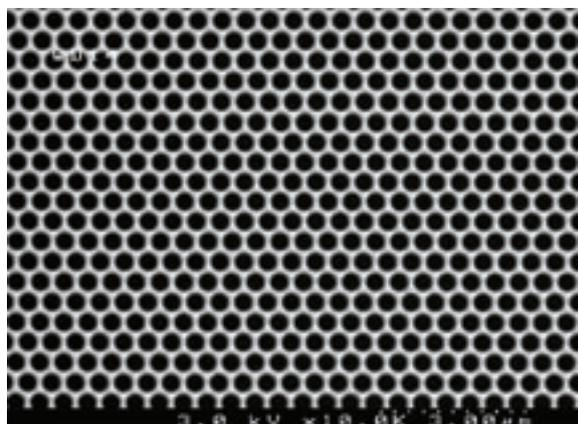
▲ A SEM image of a photonic crystal lattice milled into a 300 nm thick AMTIR-1 glass film using the FIB. The LATTICE CONSTANT is 500 nm and hole diameter 300 nm.
