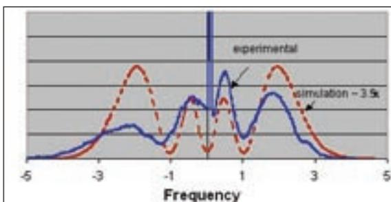
▲ Output spectrum from a 6cm long  $\text{As}_2\text{S}_3$  waveguide showing spectral broadening due to self phase modulation consistent with a nonlinear phase shift of  $\approx 3.5\pi$ . The input pulses were generated by a pulsed optical parametric amplifier seeded with a CW source which results the CW spike in the spectrum at the centre frequency.
