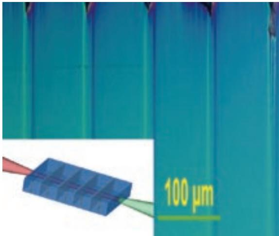
▲ Cross-sectional view of periodically poled lithium niobate fabricated using the topographical electrode technique. Inset shows a schematic illustrating frequency conversion using one of our samples.
