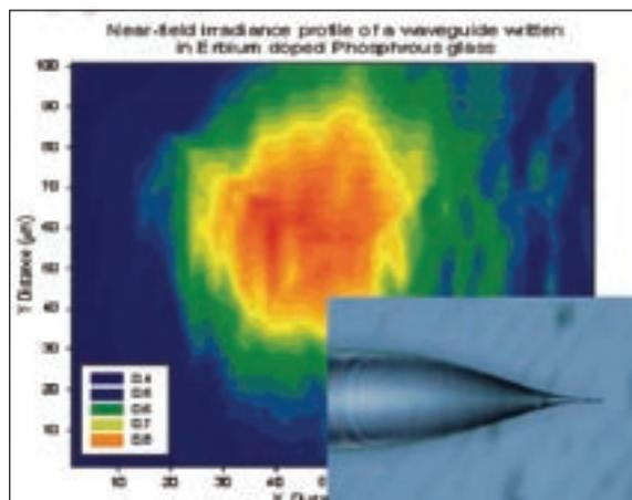
▲ False colour image of the mode field propagating through a waveguide written in erbium doped phosphate glass. This image was recorded with a tapered fibre tip (inset), with effective aperture of  $350 \text{ nm}$ , using near-field scanning optical microscopy (NSOM).
