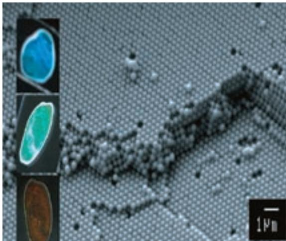
▲ Electron micrograph of a self assembled polymer opal with a period of 400 nm. Several bandgaps, at blue, green and red wavelengths (insets), are observed for this opal.
