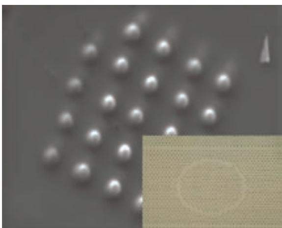
▲ Planar photonic crystal structure fabricated using micro-casting and sacrificial templates. Inset shows a planar ring resonator design generated using direct write methods.
