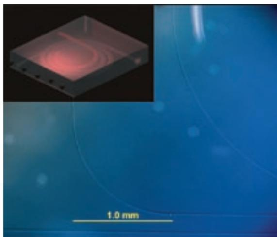
▲ Phase contrast image showing optical waveguides written inside silica using the focused output of an ultrafast laser. A conceptual view of our goal, an ultra-compact waveguide amplifier, is shown in the inset.
