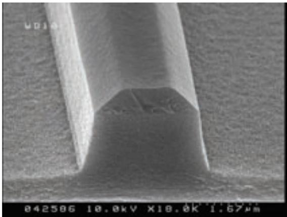
▲ SEM micrograph showing the profile of  $\text{As}_2\text{S}_3$  waveguides etched by ICP using a photoresist mask.
